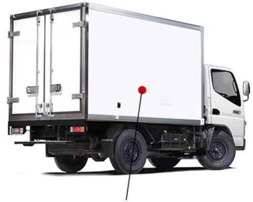
Sensor Installed in refrigerated box
